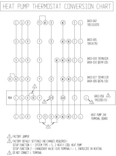
The thermostats listed below are being replaced with the 8403-058 (TH5220D1151). See the thermostat conversion charts below for any variations in terminal configuration and wiring connections:
